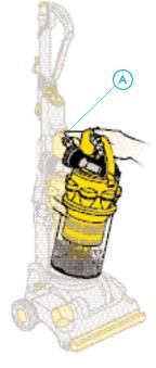
The filter may require washing more frequently than 6 months based on individual vacuuming habits. Press cyclone release button **A** to release cyclone pack.
